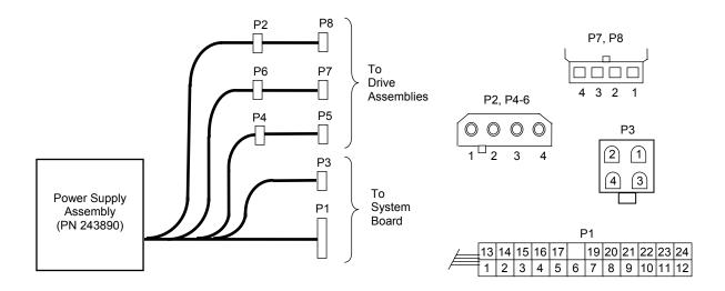
Figure 6-3 shows the cabling for the desktop and configurable minitower systems.
